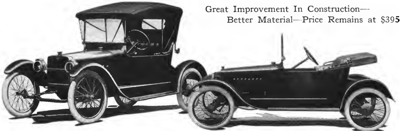
Left—Three-quarter front view of 1915 Saxon with top up and showing new streamline body. Right—Side view of new Saxon. Note running board and tank filler in cowl.
